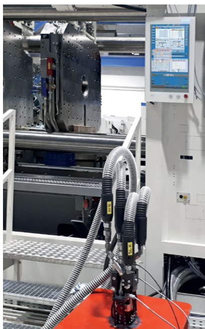
The swivel plate for the thermoplastic substrate makes the MXW 1000 from KraussMaffei particularly productive
