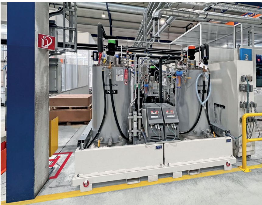
KraussMaffei supplied both the MXW 1000 injection molding machine and the RimStar Flex mixing and metering machine, including mixing heads for efficient production of components with a polyurethane surface
