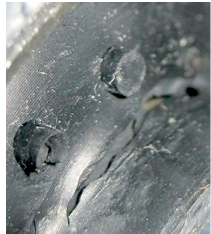
Figure 1: Cracks in a rubber part (suspension bushing) after injection molding (all pictures: SIGMA)
